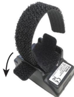
4. Remove the whole Velcro strap from the scanner by pulling the long end.
