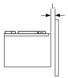
The distance between window and front of MT82VB should not exceed L=0.5mm The thickness of the window should not exceed 1mm
